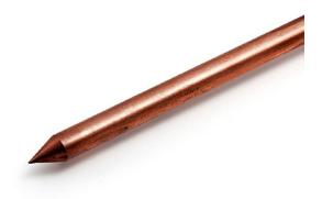
Taper pointed air rod are manufactured from electrolytic copper grade, one side taper pointed and other side with suitable threads for fixing to multi points. Rods made of aluminum can be supplied against specific requirements. Taper pointed air rod can be installed with or without multi points but use of multi points with taper pointed air rods are more effective than taper pointed air rods.
