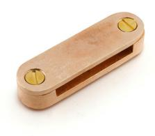
CD Tape Clip are made of gun metal or brass. The clip has a hole in the base for fixing with building or strucures with appropriate screw and well plug. These are used to secure copper tape to the building or structure.
