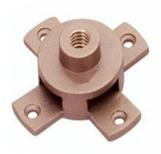
Air Terminal tape base are made of gun metal or brass. Used for vertical support to lightening conductor air terminal on the roof and flat surface. These are used for fixing air rod and connecting to tape.
