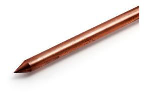
Taper pointed air rod are manufactured from electrolytic copper grade, one side taper pointed and other side with suitable threads for fixing to multi points. Rods made of aluminum can be supplied against specific requirements. Taper pointed air rod can be installed with or without multi points but use of multi points with taper pointed air rods are more effective than taper pointed air rods.
