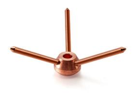
Multi point mostly used with taper pointed air rod. Multi point installed at highest area of structure or building. Multi point are mostly made of copper. Also available in brass & gun metal. Multi point also connect taper pointed air rod with elevation rod.
