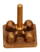
These Plates when used in concrete structures offer convenient ground system connection points. They are used where reinforcing bars are electrically continuous and are to be used as down conductors. These earth points allow easy access for the lightening protection and earthing system. Ground plate connection result in current carrying capacity equal to that of the conductor or stud and can not loosen or corrode.
